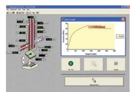
**Melt fracture/flow instability** Accelerated shear rate ramp with continuous monitoring of the pressure to detect flow instabilities, such as melt fracture which may occur during flow through a capillary die.
